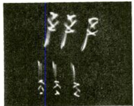
Fig. I. A 3-cycle motion of the vibrator—signals in-phase.
